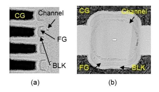
Kioxia Develops New 3D Semicircular Flash Memory Cell Structure "Twin BiCS FLASH"
